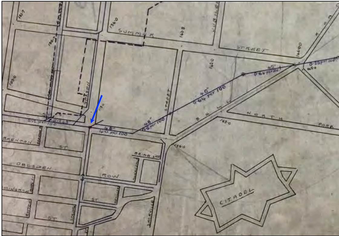
Figure 3.2-9: A 1904 map of part of Halifax shows a 48" conduit running down South Park Street to the intersection of Spring Garden (blue), north at right. 55 Here, the conduit seems to branch with one line running east down Spring Garden and another running south beside Victoria Park.
